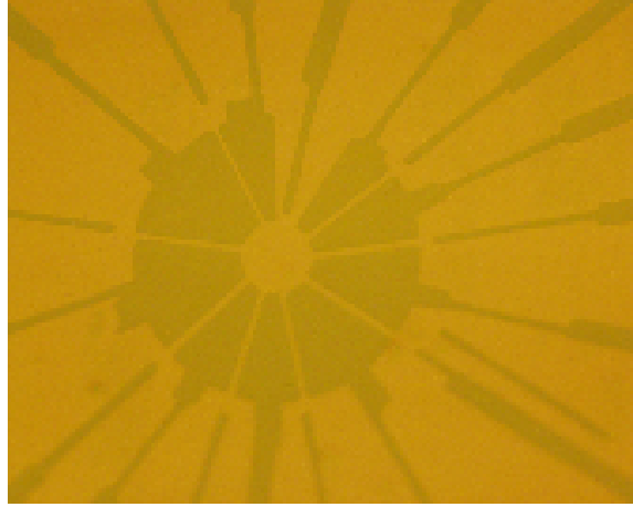
Figure 4.1: Anisotropic pattern on the YBCO film (covered by the photoresist as protection)
